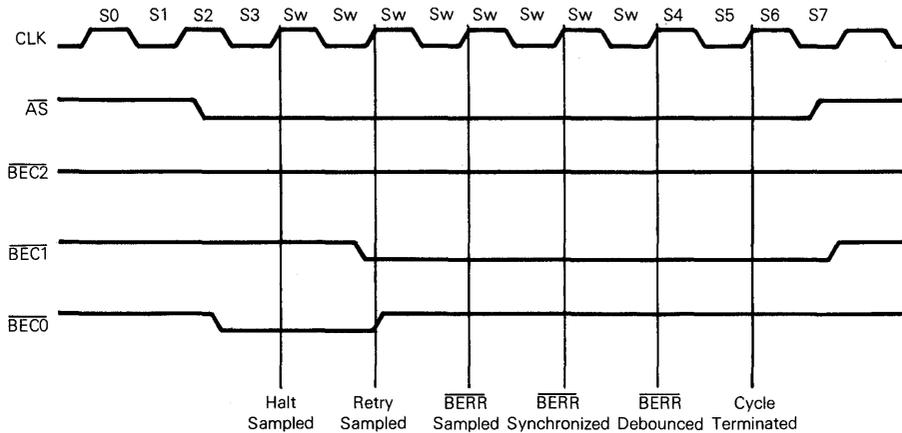
Figure 4-13.  $\overline{\text{BEC}}$  Debouncer Timing Diagram
