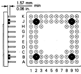
**Figure 7-1. 68-Pin Grid Array
