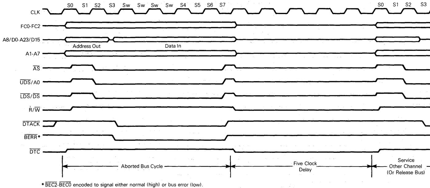
Figure 4-15. Bus Error Operation Timing Diagram
