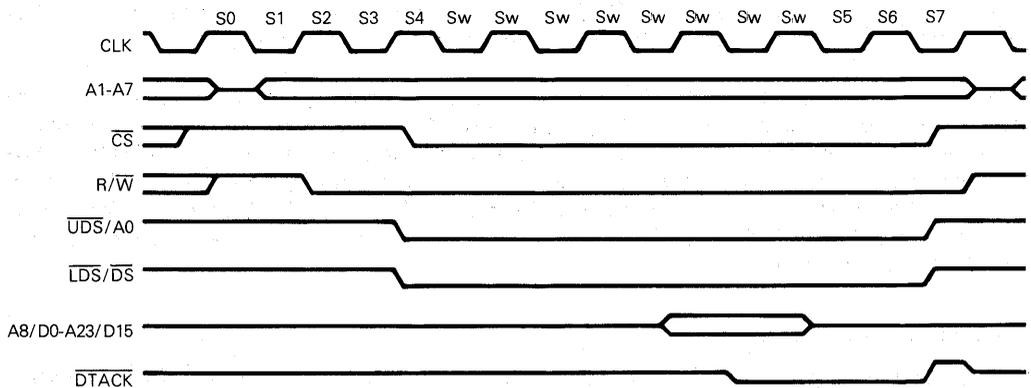
Figure 4-4. MPU Write Cycle Timing Diagram
