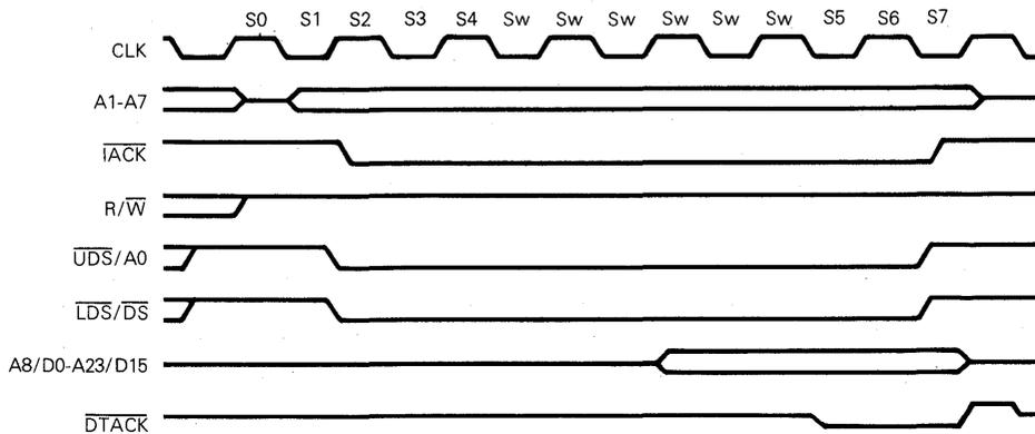
Figure 4-5. Interrupt Acknowledge Cycle Timing Diagram
