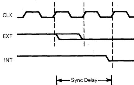
Figure 4-1. Relationship Between External and Internal Signals
