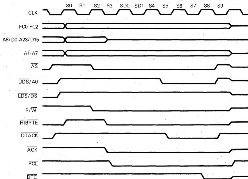
Figure 4-9. Single Address Write Cycle Timing Diagram
