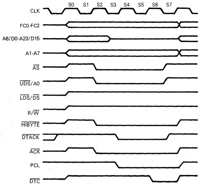
Figure 4-8. Single Address Read Cycle Timing Diagram
