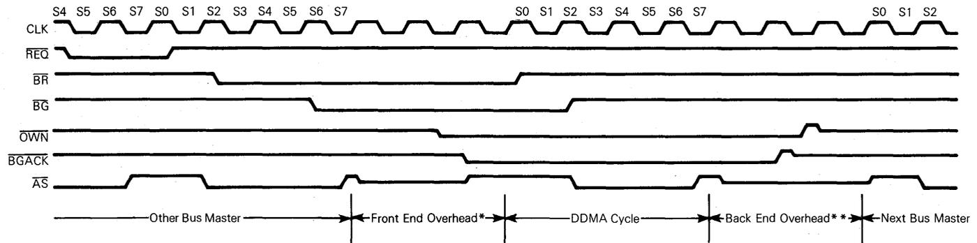
\*The front end overhead will be one clock cycle less than shown if only one channel is active.
