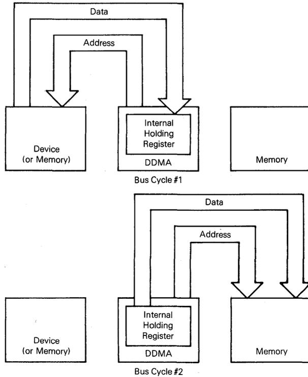
**Figure 1-4. Dual-Address Transfer Sequence**
