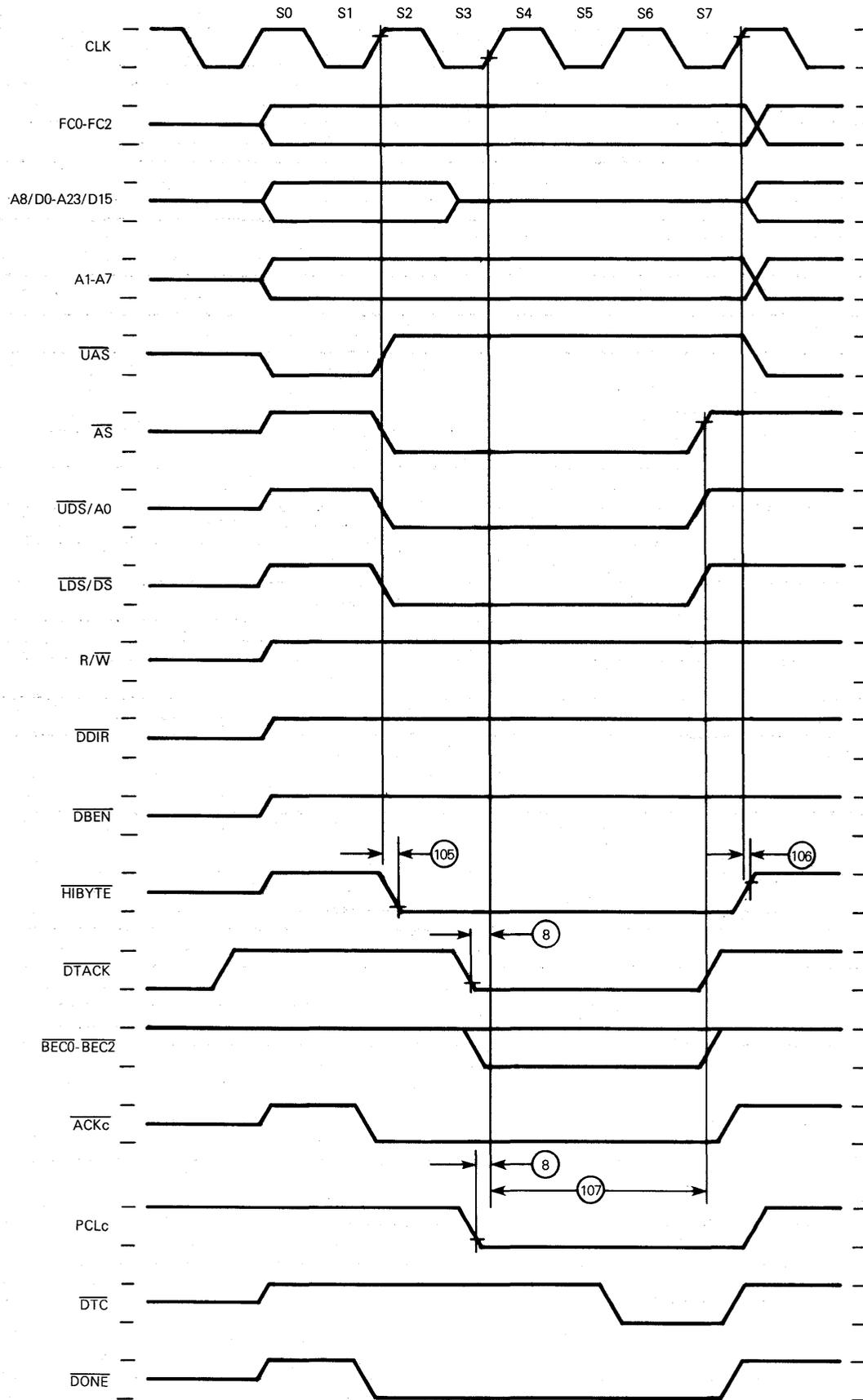
Figure 6-9. Single Address Read Cycle Timing Diagram
