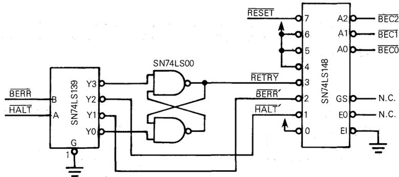
Figure 4-11. Example  $\overline{\text{BEC}}$  Signal Generation Circuit
