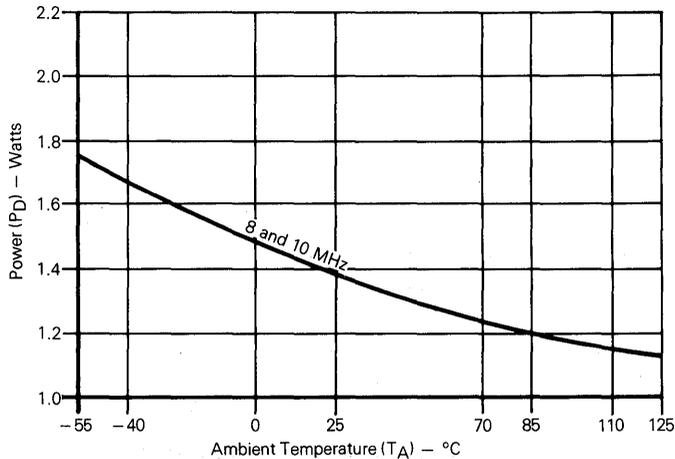
Figure 6-2. MC68440 Power Dissipation vs Ambient Temperature
