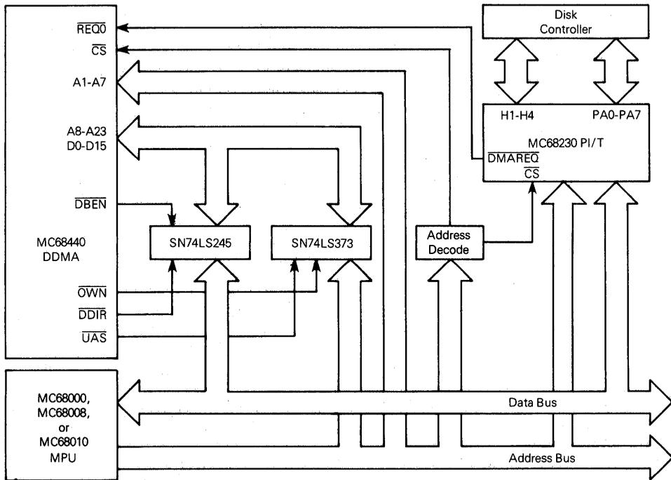
Figure 1-1. Typical System Configuration
