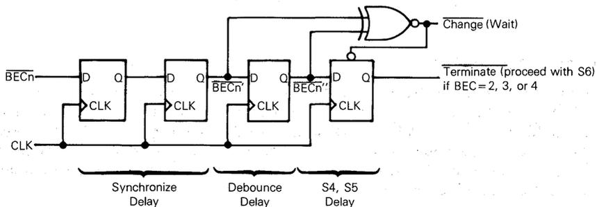
Figure 4-12.  $\overline{\text{BEC}}$  Synchronizer Functional Diagram
