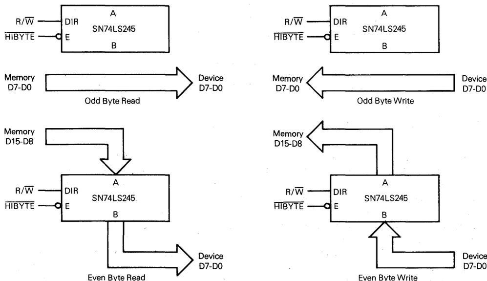
**Figure 4-10. Implicitly Address 8-Bit Device with 16-Bit Memory Data Flow**
