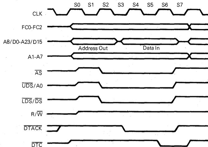
Figure 4-6. Dual Address Read Cycle Timing Diagram
