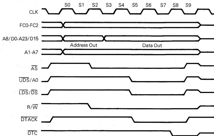
**Figure 4-7. Dual Address Write Cycle Timing Diagram**
